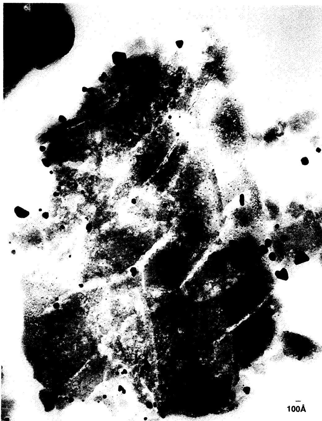
FIG. 2. Transmission electron microscopy (TEM) micrograph taken at 100 keV on a Hitachi H-600 of an ultramicrotomed section of \sim 3\% Pt/HY. When the initial calcination step is too rapid, a bimodal distribution of Pt crystallites results as seen here for the encapsulated (10–20 Å) and unencapsulated (30–200 Å) Pt particles.
