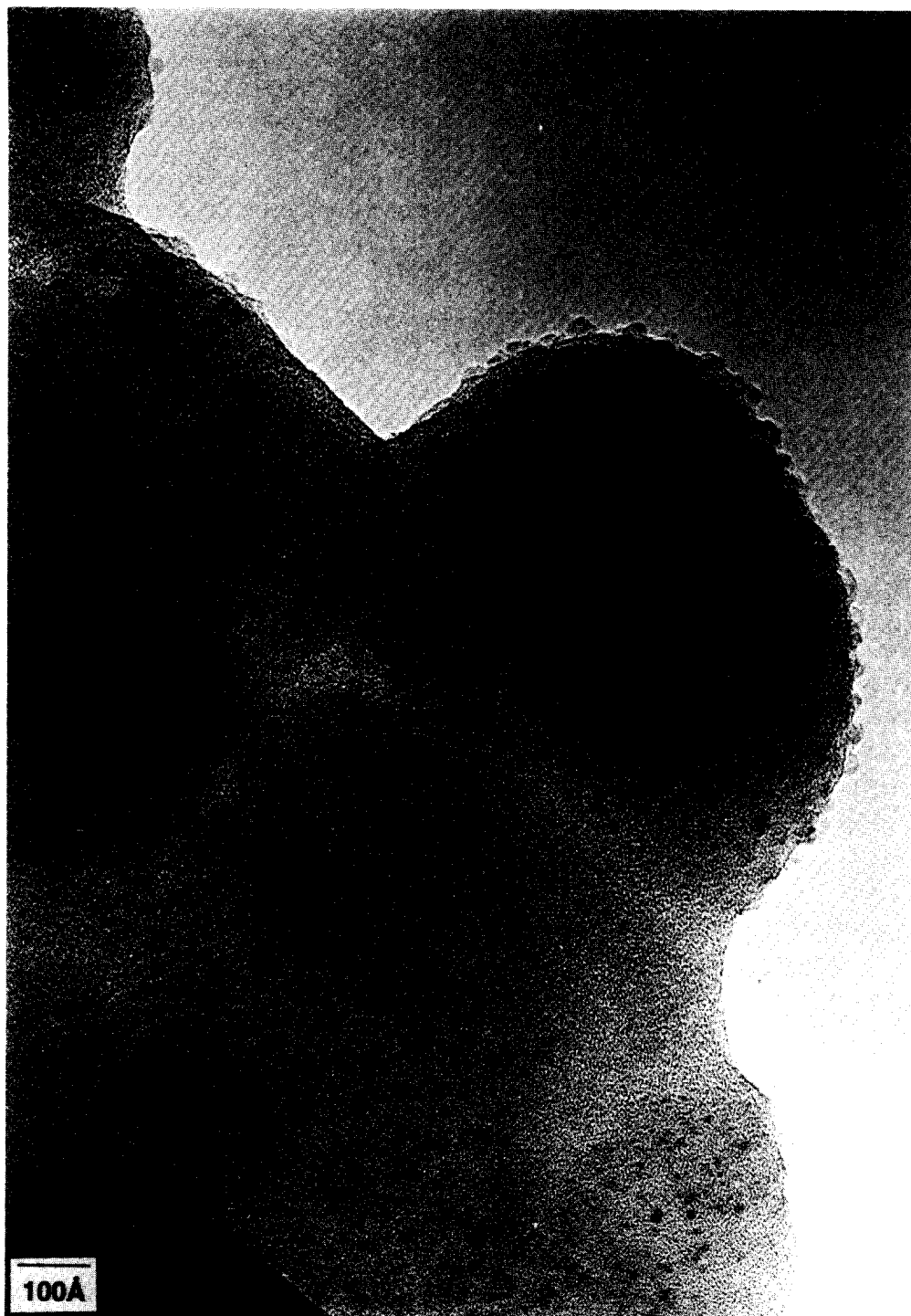
FIG. 4. TEM micrograph taken at 200 keV on a Hitachi H-800 of well-encapsulated 3.57% Pt/H-MOR showing spherical-shaped Pt crystallites of 6 to 15 Å.
